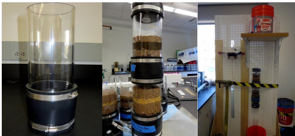
Figure 4.14: From Left to Right- One Empty Module, Two Modules Connected by Rubber Couplings, Configuration Connected to Reservoir and Ready for Testing
