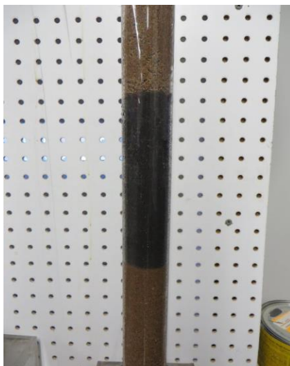
Figure 4.12: Column Test for ZVI Filings
